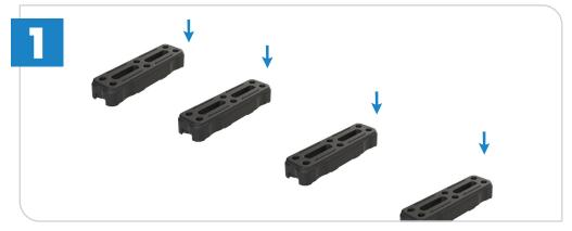
Position the rubber feet barriers along the desired perimeter line.
